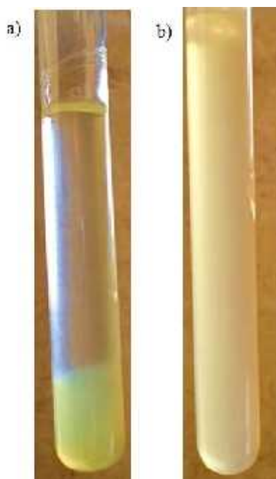
Figure 1 Suspension of 5 wt.% organoclay/acrylic dispersions: a) after 90 min mechanical agitation, and b) after 90 min mechanical agitation and 1hr sonication.
