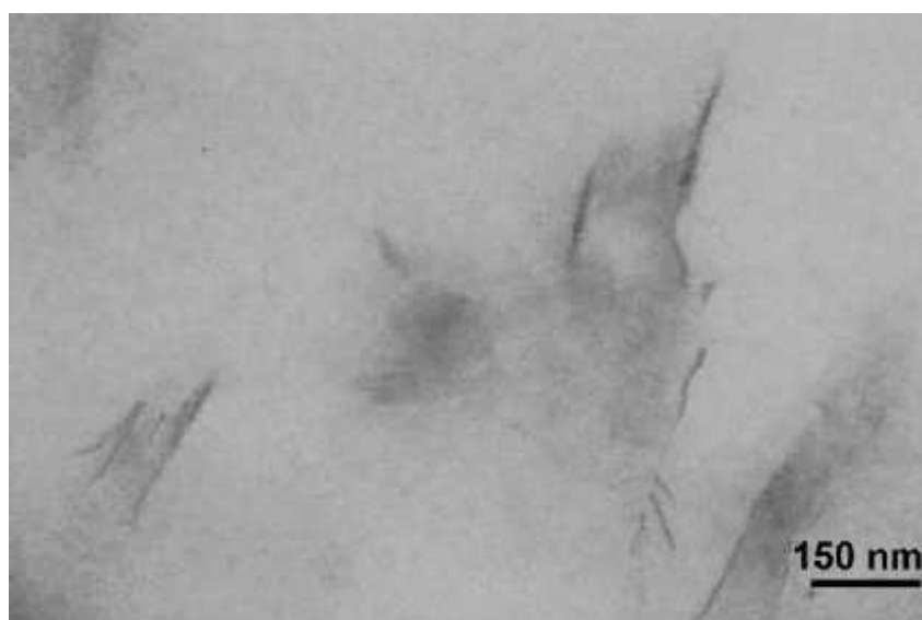
Figure 4 TEM micrographs of acrylic/3 wt.% clay nanocomposite.
