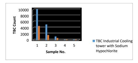
**Figure 6**Comparing the TBC results obtained from the performance of sodium hypochlorite and hypochlorous acid in an industrial cooling tower in the same period.
