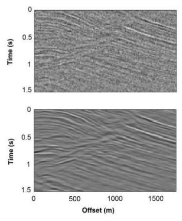
**Figure 5**a) The close-up of a part of noisy seismic section containing an event like fault before denoising; b) the zoom of noisy seismic section after denoising by FXD+DBM; the high ability of combination strategy to improve the S/N ratio and interpretability of the section in comparison to the simple method is clear.
