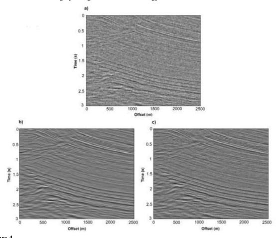
**Figure 4**a) A real noisy seismic section; b) the denoised seismic section by FXD+DBM; c) the denoised seismic section by FXD; from the results, after denoising, the SNR is improved using both approaches, but FXD+DBM method shows higher performance.
